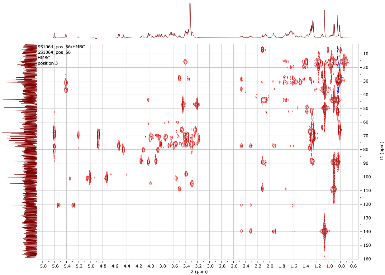
Figure S37. gHMBCAD NMR spectrum for the intact molecule of the switchgrass saponin SS1064.
