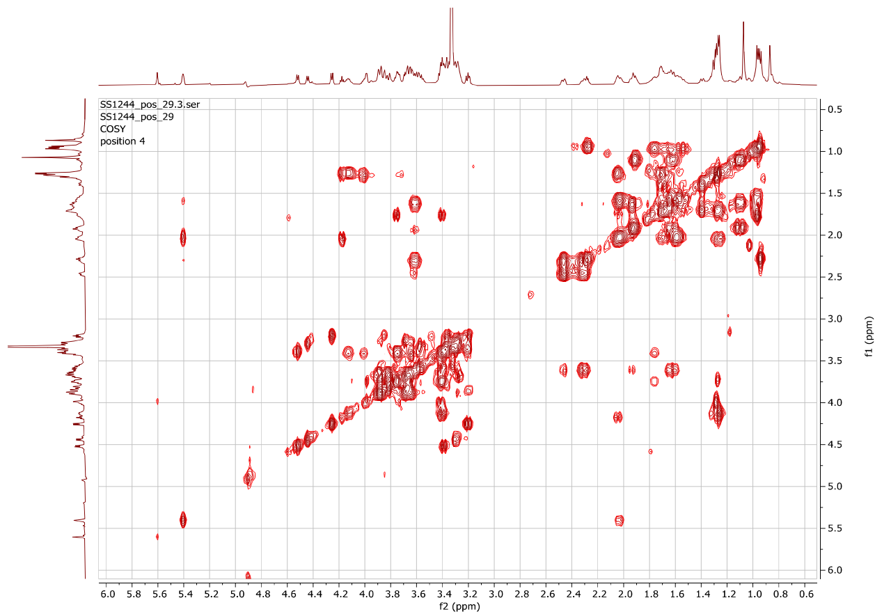
Figure S29. gCOSY ^1\text{H} - ^1\text{H} NMR spectrum for the intact molecule of the switchgrass saponin SS1244.
