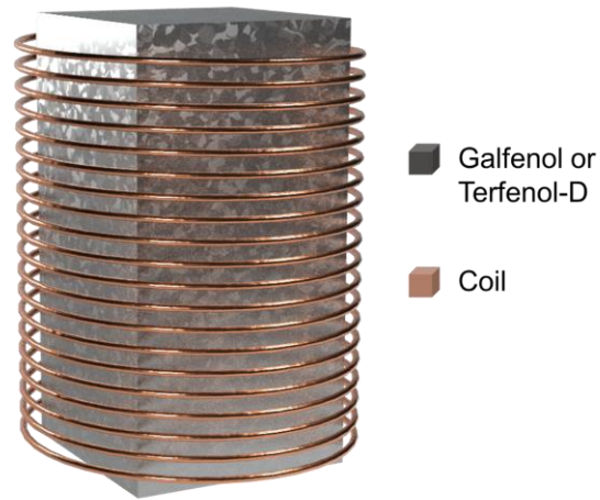
Figure S2. Conventional magnetoelasticity system based on the rigid Galfenol or Terfenol-D for mechanical-to-electrical conversion. Rigid magnetoelastic materials such as the Galfenol or Terfenol-D can be deformed by external pressure and generate the magnetization variation. 2,3 The corresponding magnetic flux density change will induce an electromotive force in the rigid coils based on Faraday's law of induction.
