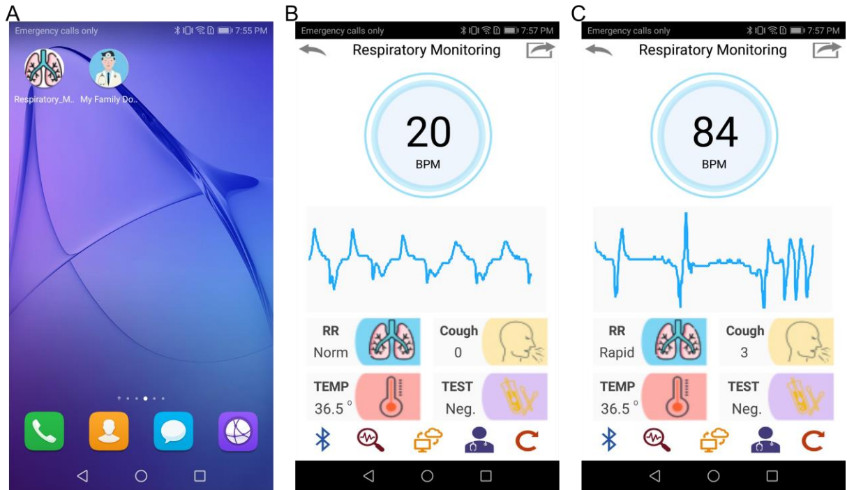
Figure S17. Customized cellphone APP for respiratory monitoring data display.
