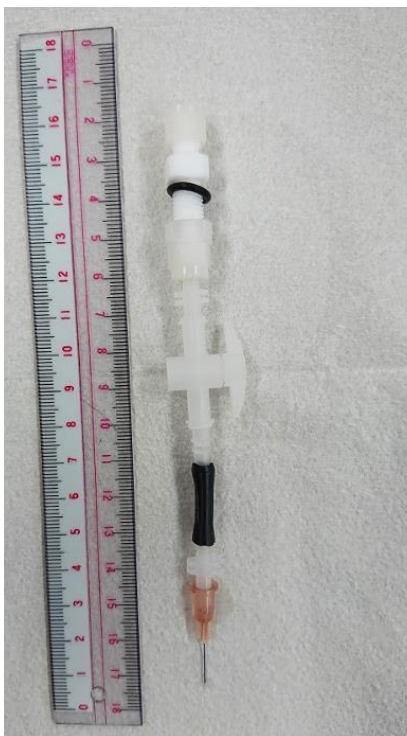
Figure S2. Apparatus used in semi flow-through water renewal system. A) Needle and connecting tube. B) Exposure glass beaker with a 6.7 mm (i.d.) hole. C) Stainless-steel mesh (opening size: 500 \mu\text{m} ), screw, and nut to cover an overflow hole of glass beaker.
