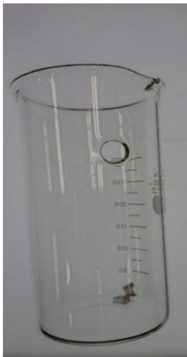
Figure S2. Apparatus used in semi flow-through water renewal system. A) Needle and connecting tube. B) Exposure glass beaker with a 6.7 mm (i.d.) hole. C) Stainless-steel mesh (opening size: 500 \mu\text{m} ), screw, and nut to cover an overflow hole of glass beaker.
