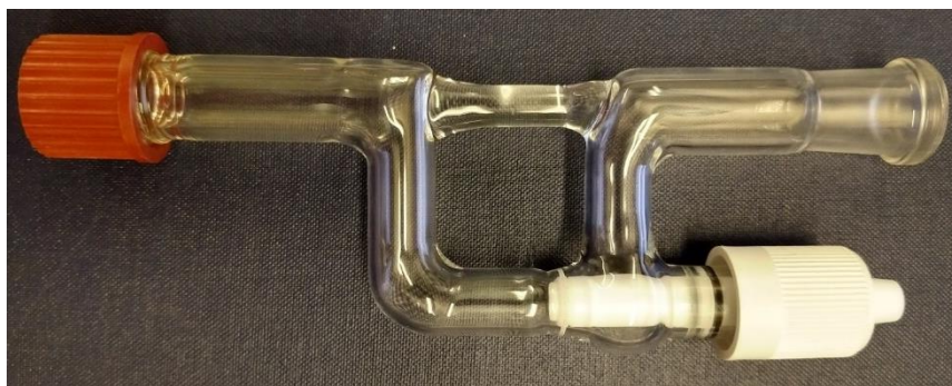
Figure S1. Reusable adapter to seal NMR tubes for samples in high boiling point solvents. This adapter has been developed by Elijah Aller.
