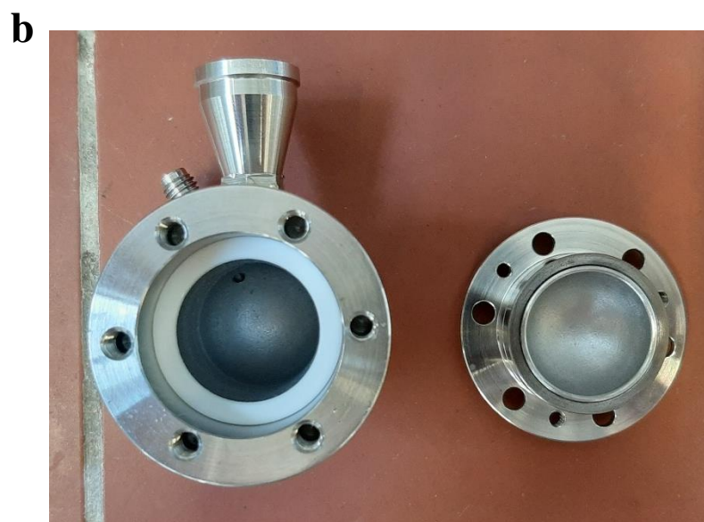
Fig. S7: Further details of the home-built pressurizable milling jar. a) Technical drawing (cross section) of the jar, showing the gas inlet (1) with brass sealing and metal frit. b) Picture of the jar, body (left) and lid (right).
