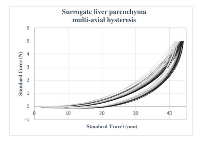
**Supplementary file 5.** The hysteresis curves for PDMS A10 with 300% oil surrogate liver resulted in an accurate characterisation of the ultimate tensile strength (UTS). Vectors in this graph show force (N) versus travel (mm) for five different specimens during multi-axial compression up to a maximum of 5N.
