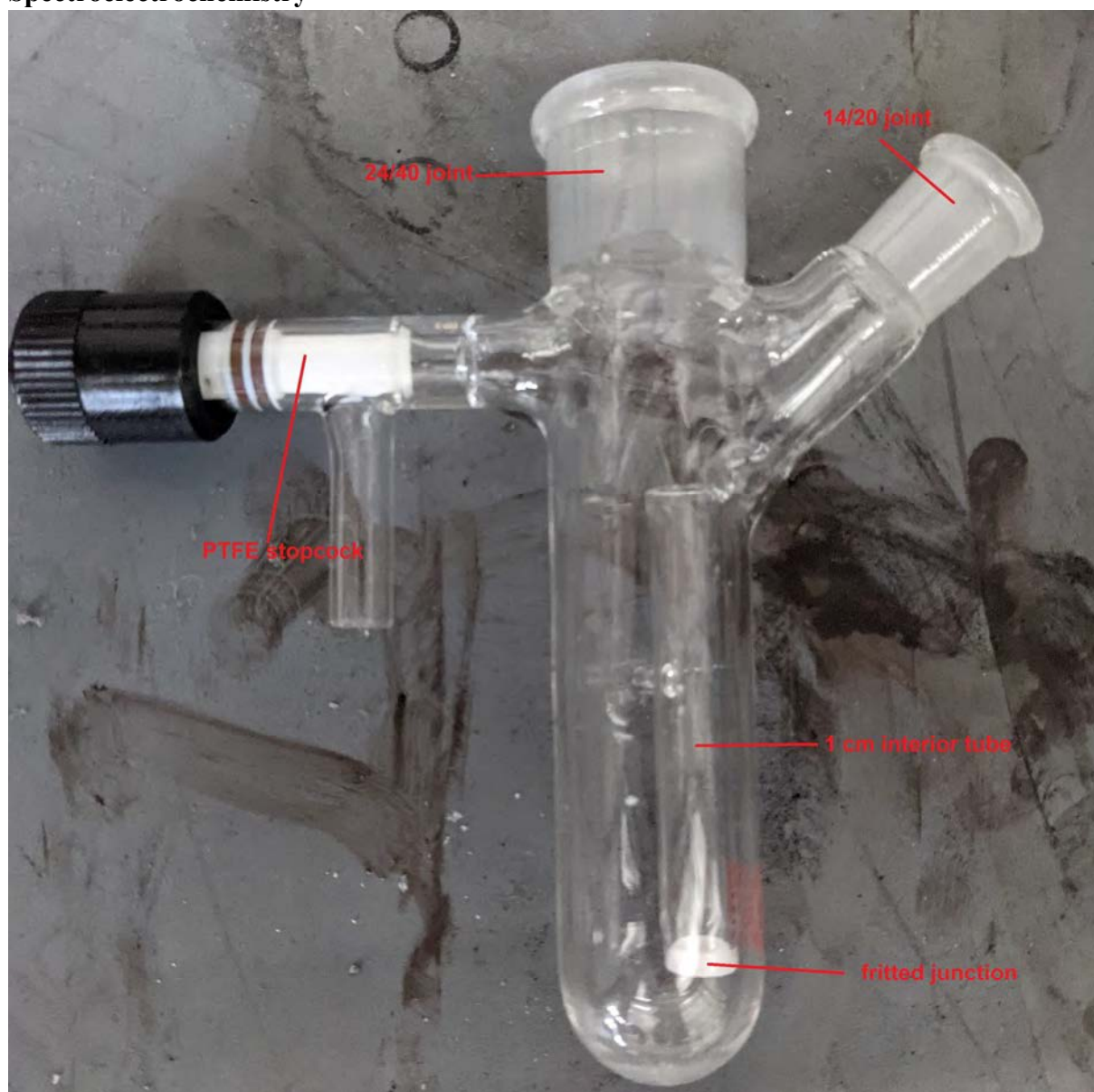
Schlenk-type divided cell apparatus used for spectroelectrochemical experiments.
