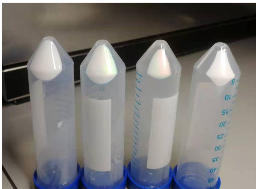
Figure S14. Photograph of the self-assembled superstructures resulting from the centrifugation of different aqueous colloidal MOF particles (from left to right: RD-ZIF-8, TRD-ZIF-8, C-ZIF-8 and O-UiO-66). Strong iridescence is observed for TRD-ZIF-8 sample. Weak iridescence is observed for C-ZIF-8 sample. No color is observed for RD-ZIF-8 and O-UiO-66 samples.
