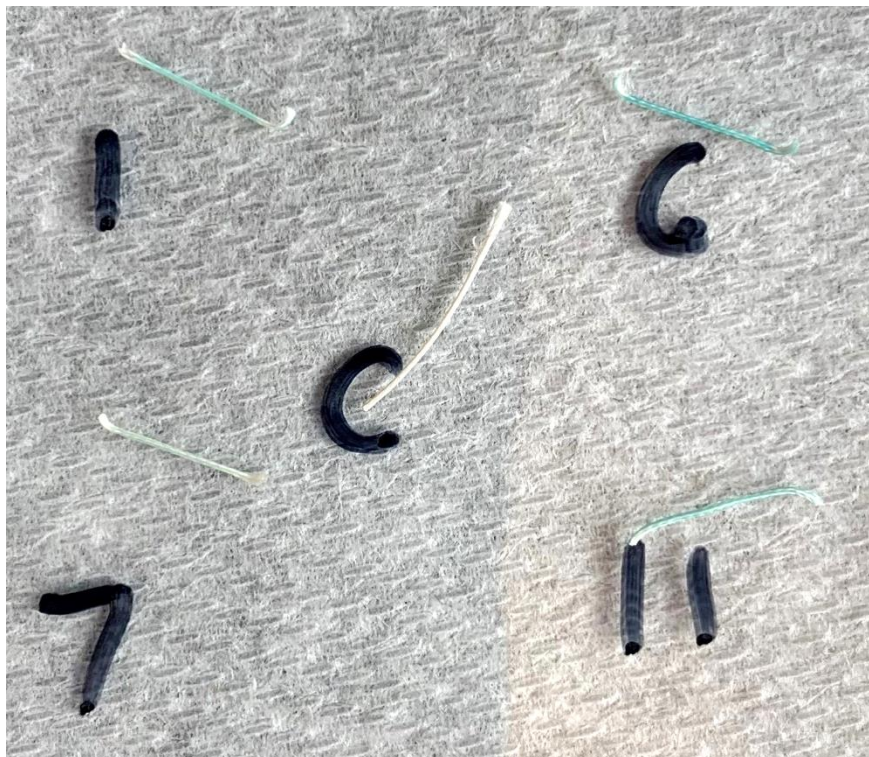
Figure S7. Digital imaging of fluorescently labeled siRNA sutures. siRNA-coated LbL sutures using an AlexaFluor647 labeled control siRNA were imaged and compared to an uncoated suture (C). Representative pieces of suture from 4 sets of solution conditions (1, 6, 7, and 11) are demonstrated. Blue color is indicative of the amount of fluorescent siRNA loaded onto the suture.
