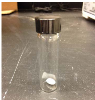
Step 1: Flame dried 2-dram vial and stir bar
