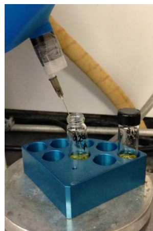
Step 4: Sparge degassing technique with argon balloon and 4" hypodermic needle
