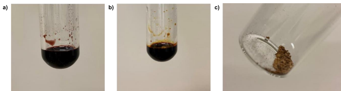
Figure S3. Photographs of the vials (a) before and (b) after microwave-heating process and (c) the final CNDs-2 after precipitation in cold \text{Et}_2\text{O} and subsequent filtration.
