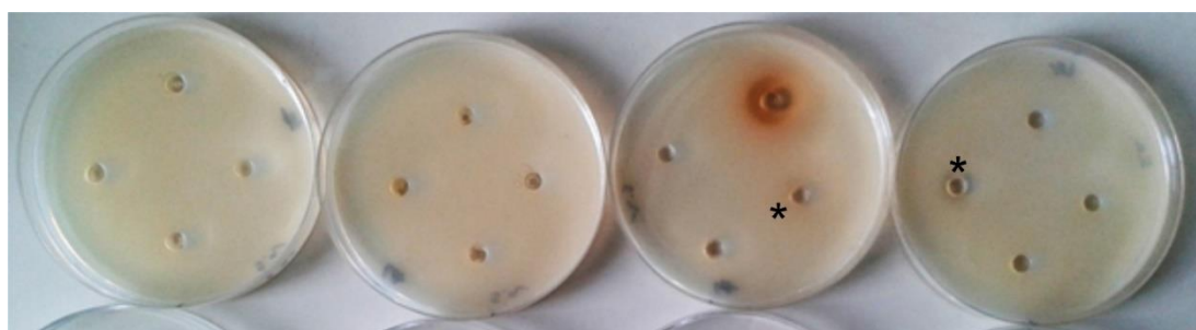
Figure S1. Representative photograph of the agar diffusion assay using S. aureus NCTC 6571 where a selection of different myxocoumarin derivatives was dissolved in DMSO (50 mg/mL) and 5 µL (250 µg of compound) was added to each well. Asterisk mark the zones of clearance, after 24-h incubation period.
