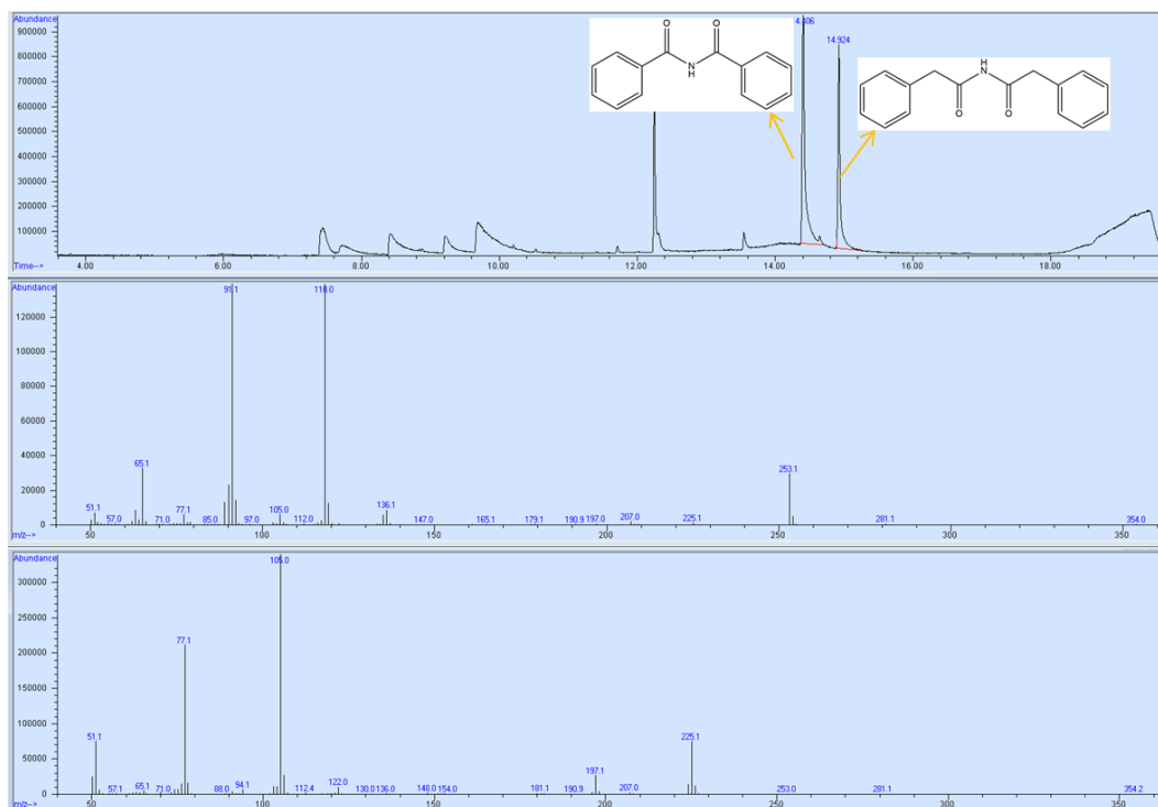
Figure S36. GC-MS data of reaction solution for the (0.045 mmol) reacts with phenylacetyl chloride (0.18 mmol) after drying treatment of molecular sieve for 24 hours. Theoretical m/z of 2-phenyl-N-(2-phenylacetyl)acetamide: 253.1; experimental m/z of 2-phenyl-N-(2-phenylacetyl)acetamide: 253.1. The yield is calculated as 72% based on the amount (33 \mu mol) of 2-phenyl-N-(2-phenylacetyl)acetamide calculated from its ratio of integral peak area relative to signal peak of internal standard (N-benzoylbenzamide) in the GC-MS chromatogram.
