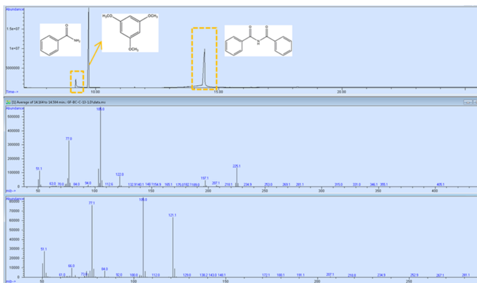
Figure S29. GC-MS data for the reaction mixture solution obtained by mixing \text{Li}_3\text{N} (0.06 mmol) with one equivalent of benzoyl chloride (0.06 mmol). Theoretical m/z of 2a N-benzoylbenzamide: 225.1; experimental m/z of 2a N-benzoylbenzamide: 225.1. Theoretical m/z of 1a benzamide: 121.1; experimental m/z of 1a benzamide: 121.1.
