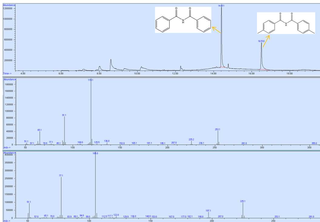
Figure S37. GC-MS data of reaction solution for the (0.045 mmol) reacts with p-toluoyl chloride (0.18 mmol) after drying treatment of molecular sieve for 24 hours. Theoretical m/z of 4-methyl-N-(4-methylbenzoyl)benzamide: 253.1; experimental m/z of 4-methyl-N-(4-methylbenzoyl)benzamide: 253.1. The yield is calculated as 69% based on the amount (31 \mu mol) of 4-methyl-N-(4-methylbenzoyl)benzamide calculated from its ratio of integral peak area relative to signal peak of internal standard (N-benzoylbenzamide) in the GC-MS chromatogram.
