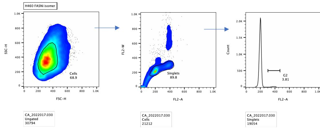
**Supplementary Figure 11. Gating strategy for cell cycle facs experiments.** Cell population is gated in SSC-H/FSC-H to remove debris (gate “Cells”). “Cells” population is then gated in FL2-W/FL2-A to select only single cells (gate “Singlets”). The “Singlets” population is represented as histogram over FL2-A. G2 peak is gated in the “Singlets”.
