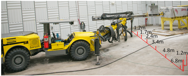
Fig. S1—Laboratory experiment setup in the NIOSH hemi-anechoic chamber.
