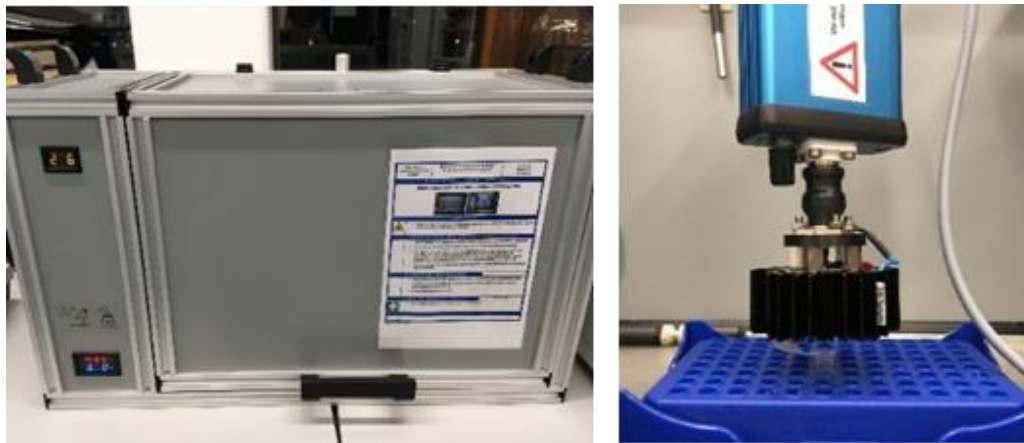
Supplementary Figure 2. LED setup used in this study. Outside of the box (left) and distance between the LED and the sample (right).
