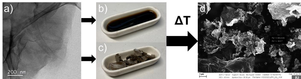
Figure S1. Comparison of two different batch approaches to the synthesis of rGO supported catalysts (a) TEM image of the GO (b) GO suspension impregnated with metal-salt precursor (c) freeze-dried GO suspension with impregnated metal-salt precursor (d) result of thermal decomposition of samples in figures (c) and (b) .
