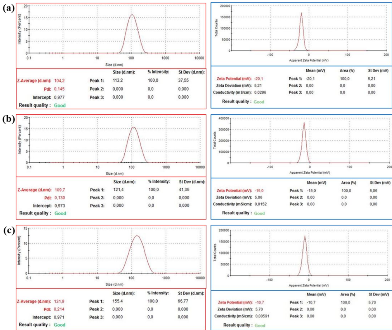
Figure S8. Distribution curves of mean size (intensity %) and zeta potential of sample Man-LPHFNPs@Roflumilast freeze-drying (a), and after freeze-drying and redispersion in bidistilled water (b) or in a 10 mM NaCl aqueous solution (c).
