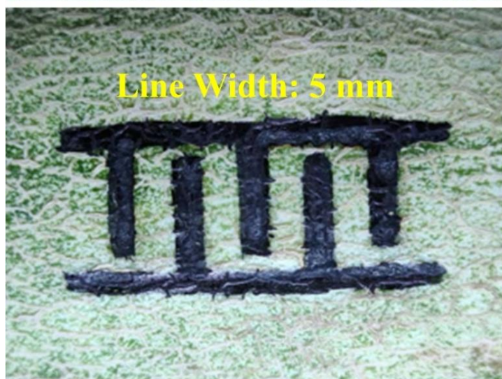
Figure S1. Photograph of graphene patterned into a shape of the interdigital electrodes on cantaloupe peels by using concentrated solar radiation. Top: 8 interdigital electrodes with a line width of ~3 mm. Down: 5 interdigital electrodes with a line width of ~5 mm.
