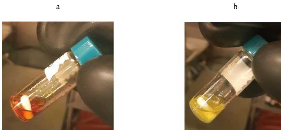
Figure S11: Pictures of solutions of FACsSnI 3 (a) with SnI 4 (b) 10% SnF 2 . The red component is an indication of the content of Sn 4+ .
