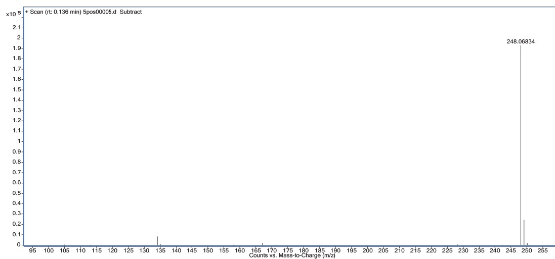
Supplementary Fig. 25 | HRMS of CZA. (\text{CzA}+\text{Na})^+ m/z: 248.0683 (theoretical value: 248.0687).
