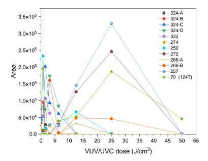
**Fig. S1** Transformation products of aqueous TEB samples identified by LC-HRMS after VUV irradiation. Transformation products are denoted by their mass-to-charge (m/z) ratio. 124T refers to 1,2,4-triazole.
