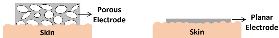
Figure S3. Schematics illustrating the difference in skin-electrode contact area between the porous electrode and planar electrode when no conductive hydrogel is used.
