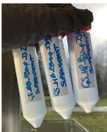
Figure S7. PB milled, tip sonicated and centrifuged EB-NS, HB-NS and HP-NS Self-taken photograph of the fully exfoliated samples, i.e. the final NS batches that underwent complete morphological and photophysical characterization.
