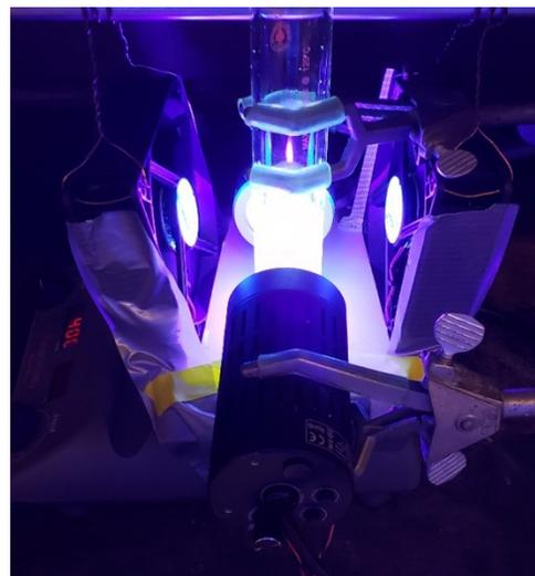
**Figure S6.** Gram-scale synthesis using 2 Kessil<sup>®</sup> LEDs at 100% power with 2 fans facing each other for cooling
