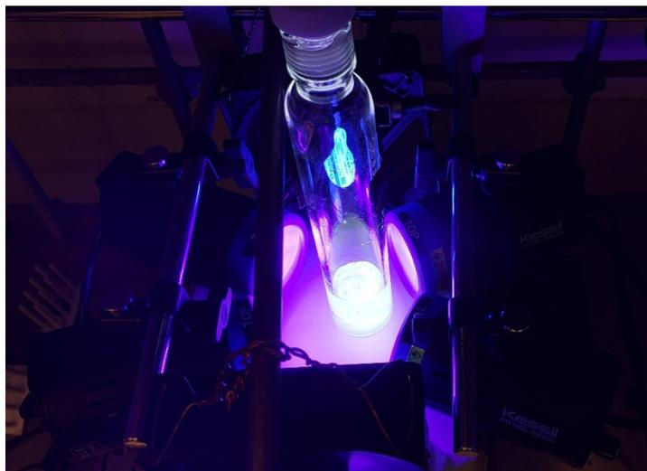
**Figure S5.** Gram-scale synthesis using 4 Kessil<sup>®</sup> LEDs at 50% power with 2 fans facing each other for cooling
