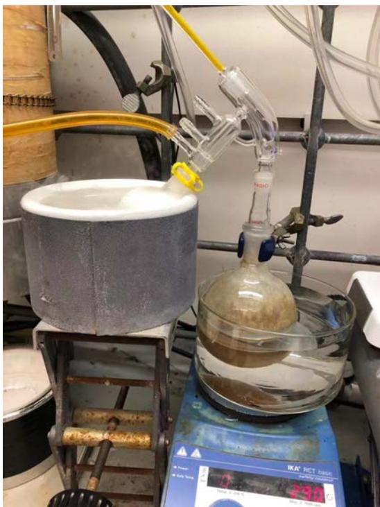
Figure S2. Distillation set-up
