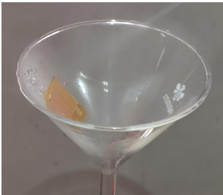
Figure S18. Optical image showing condensed droplets sliding over the condensate energy harvester attached to a curved surface. The condensate energy harvester is made of a SLIPS layer and a flexible printed circuit board integrated with transistor-like electrode architecture.
