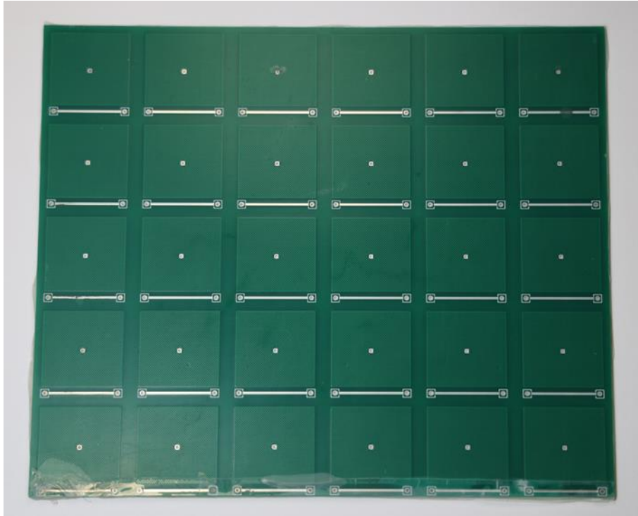
Figure S21. Optical images of the wave energy harvester consisting of 6×5 pieces of LA-TEGs.
