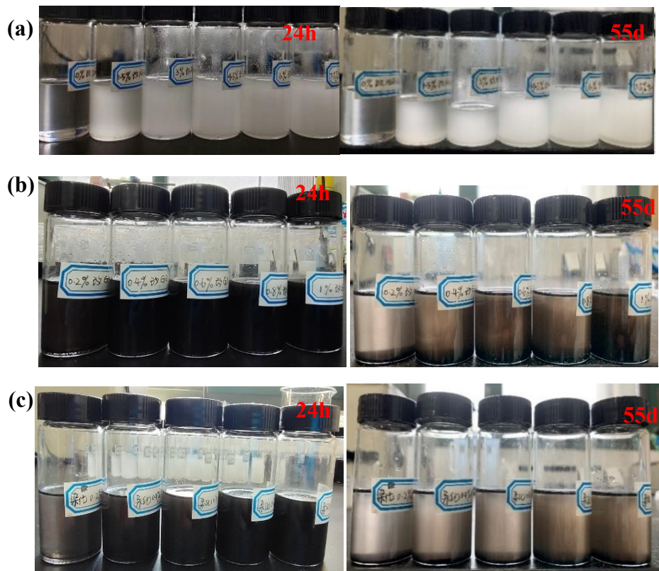
Figure 5S Dispersion and stability of nanoparticles with different contents in epoxy resin for different holding times, (a) m-Al 2 O 3 (b) mGO and (c) m-Al 2 O 3 @GO hybrids
