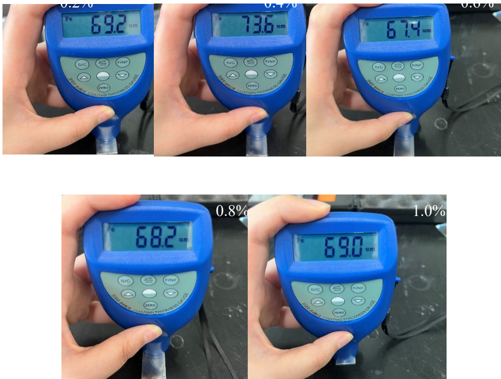
Figure 1S The thickness of the composite coatings, (a) the neat epoxy coating and m-Al 2 O 3 /epoxy coating, (b) mGO/epoxy coating and (c) m-Al 2 O 3 @GO/epoxy coating
