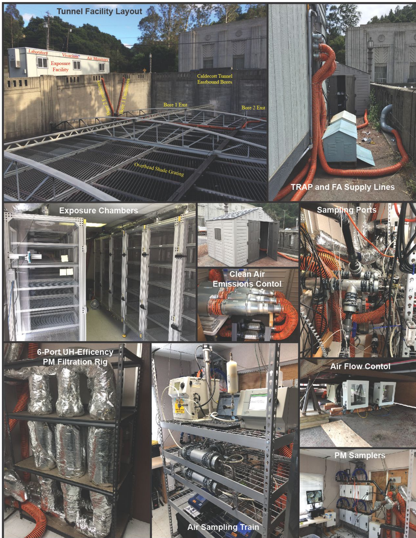
Figure S1. Photo montage of the various systems comprising the Caldecott Tunnel Exposure Facility (CTEF). S3
