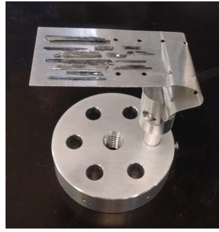
Figure 4. CrSBr sample used for the neutron experiment, consisting of 13 coaligned crystals glued to an aluminum plate for a total mass of 300 mg. The c axis is vertical, and the longest crystal edge is along the a axis.
