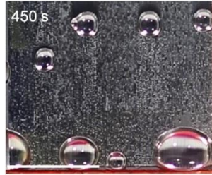
Fig. S23. Condensation on hydrophilic reentrant SLIPS with a spin speed of (A) 2000 rpm with droplet emergence due to low pinning force, and (B) 8000 rpm. The scale bar is 5 mm.
