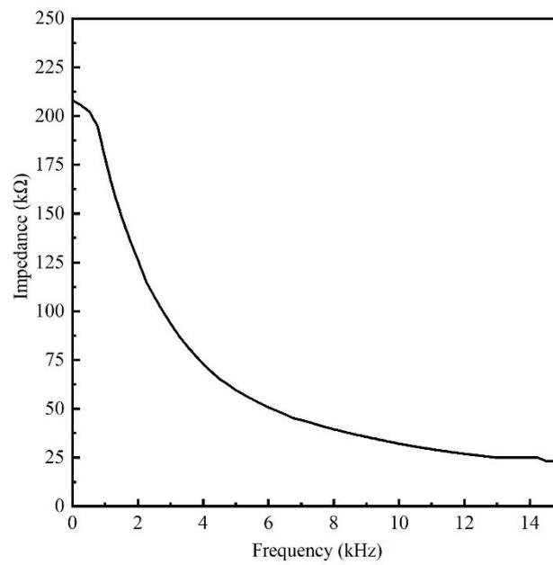
**Fig. S1. The impedance of human fingertip skin with stimulation current frequency.** The positive electrode is located in the center of the fingertip, and the negative electrode is four adjacent electrodes connecting. The electrode is a half-spherical-shaped bump with 1 mm radius.
