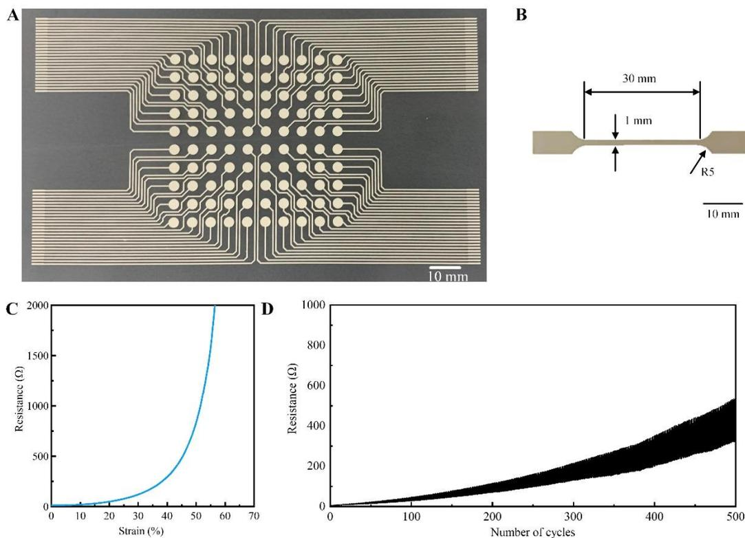
**Fig. S11. 10×10 stretchable TPU-based electrode array.** (A) The optical image of 10×10 stretchable TPU-based electrode array. (B) The optical image of test sample. (C) Resistance response of the test sample under the uniaxial tensile strain. (D) Cycle tests of the sensor with 500 cycles of repeated stretching to 10% strain.
