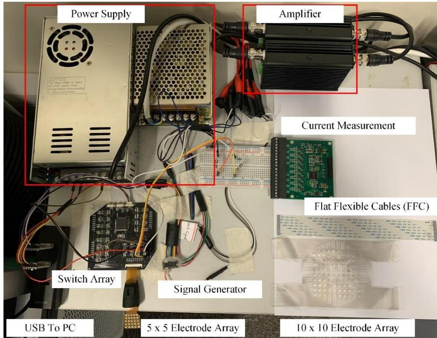
**Fig. S3. Optical image of all electro-tactile devices.** The signal generator is controlled by the computer software to generate the specified waveform. The signal is amplified by the power amplifier as the input signal of the switch array circuit board. The switch array circuit board is connected to the electrode array through the FFC and independently controls the state of each stimulation electrode. Each device is connected by wires.
