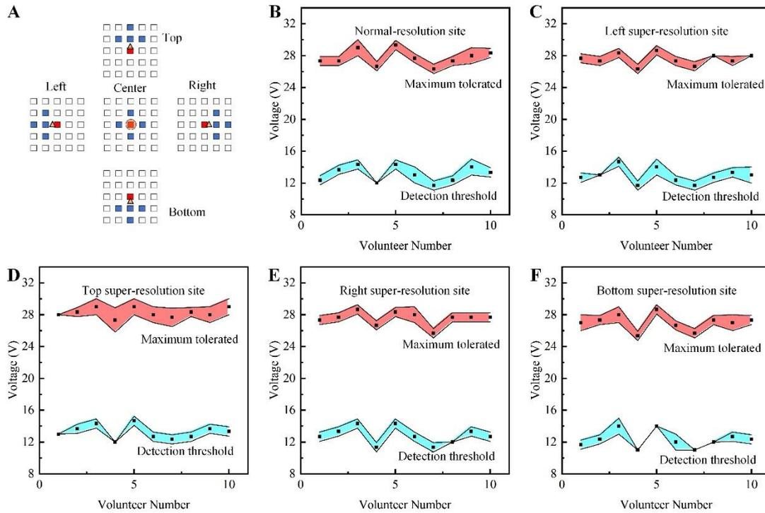
**Fig. S8. Intensity test of center normal resolution and super-resolution sites.** (A) Schematic of the distribution of stimulus electrode states. (B-F) The relationship between tactile perception intensity and stimulation voltage for five sites. Error bars indicate the fluctuation of the test results of each volunteer in multiple measurements.
