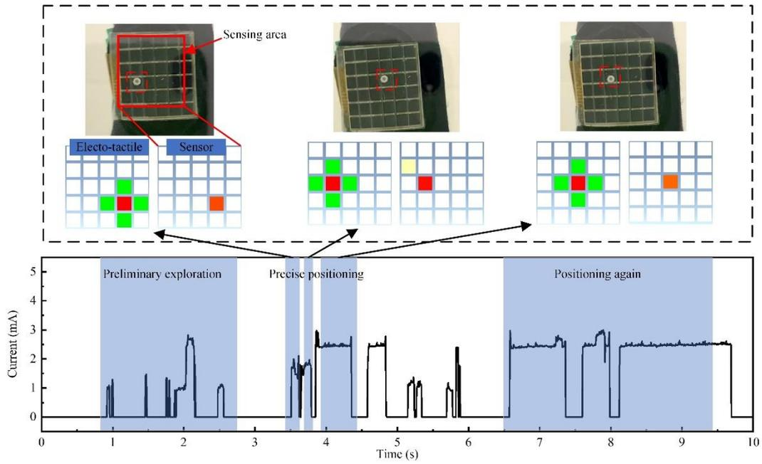
**Fig. S12.** The real-time signal of the sensor-actuator glove system. After a short preliminary exploration, the volunteer accurately positions the target at the center of the fingertips.
