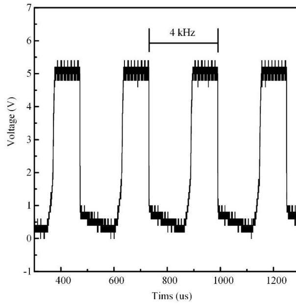
**Fig. S6. The refresh rate of stimulating electrode state switching.**
