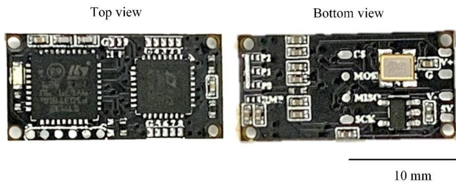
**Fig. S4. Optical image of the signal generator circuit board.**
