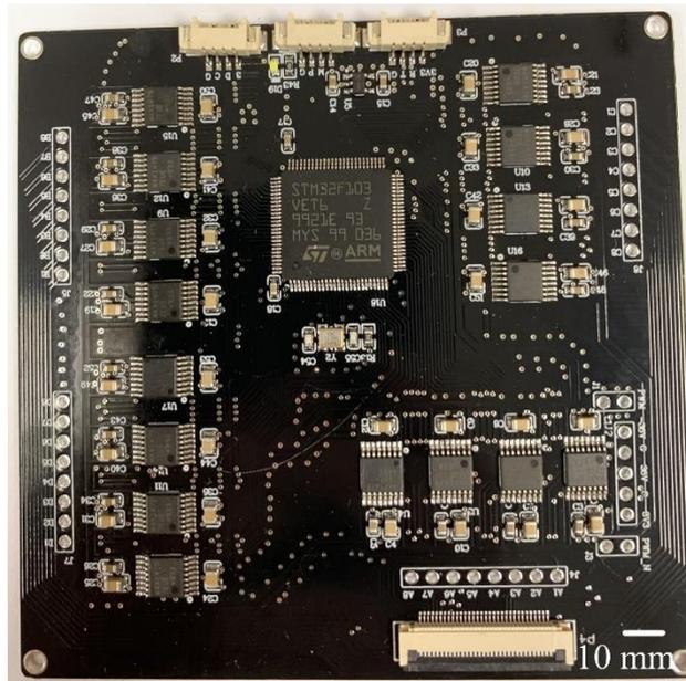
**Fig. S5.** Optical image of the switch array circuit board.
