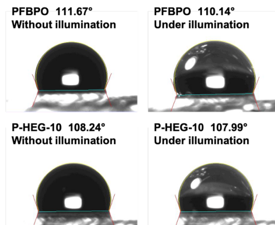
The water contact angle of polymers before and under illumination.
