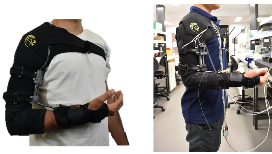
Figure 4 illustrates an example of an upper limb exosuit robot described by Hoang et al. being worn by a volunteer. *Note: The person shown in the picture is not a patient and was taken with the participant's knowledge and permission. Picture courtesy of Dr Thanh Nho Do.
