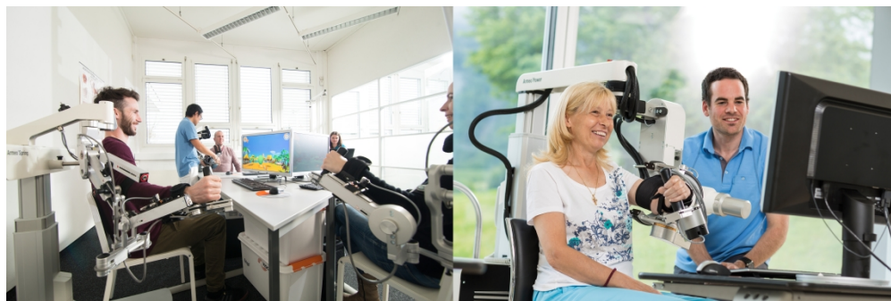
Figure 3 illustrates an example of upper limb training using an exoskeleton robot, ArmeoPower. *Note: The person shown in the picture is not a patient and was taken with the participant's knowledge and permission. Picture courtesy of Hocoma.
