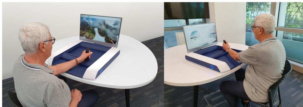
Figure 1 illustrates an example of upper limb training using an end-effector robot, H-man. *Note: The person shown in the picture is not a patient and was taken with the participant's knowledge and permission. Picture courtesy of Articares.
