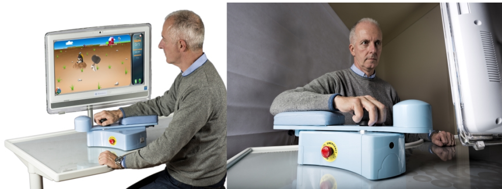
Figure 2 illustrates an example of upper limb training using an end-effector robot, MO.TO.RE. *Note: The person shown in the picture is not a patient and was taken with the participant's knowledge and permission. Picture courtesy of Humanware S.r.l.
