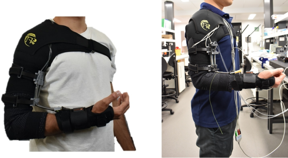
Figure 4 illustrates an example of an upper limb exosuit robot described by Hoang et al. being worn by a volunteer. *Note: The person shown in the picture is not a patient and was taken with the participant's knowledge and permission. Picture courtesy of Dr Thanh Nho Do.
