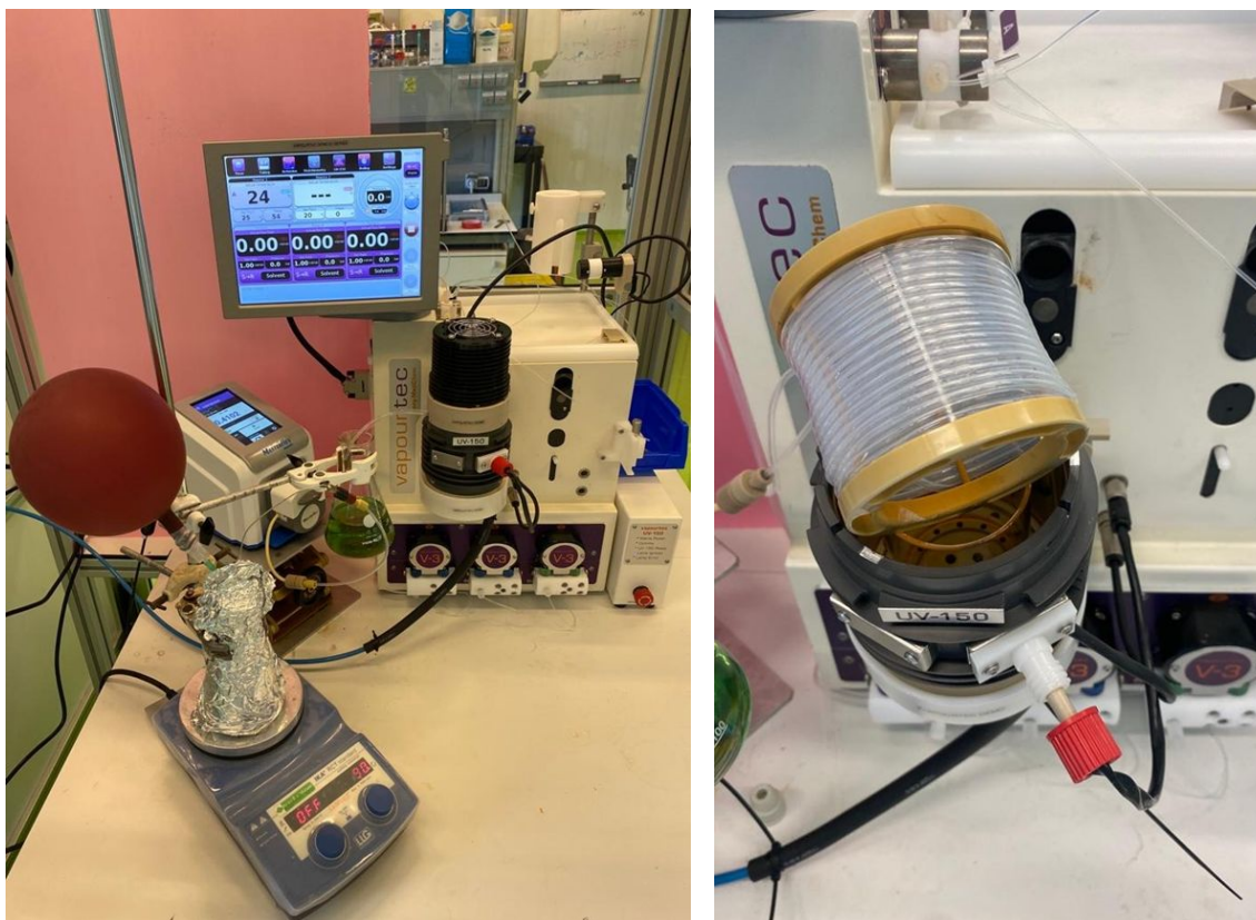
Figure S4 Overview and details of the Vapourtec system (flow setup for scale-up): in particular, PFA coil (internal diameter 2.0 mm, external diameter 3.0 mm) is shown.
