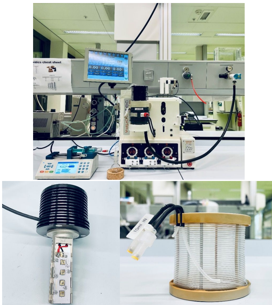
Figure S3: Overview and details of the Vapourtec system: in particular, LEDs and the PFA coil (internal diameter 1.3 mm, external diameter 1.6 mm) are shown.
