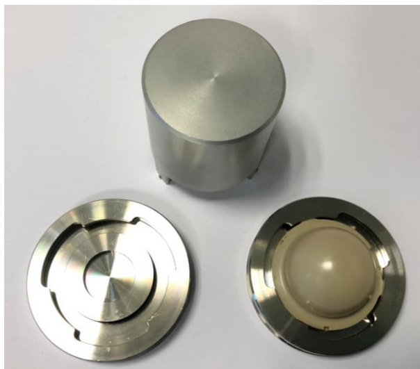
Figure S33. Digital photos of the XRD sample holder with PEEK dome used for XRD measurement without air exposure. The thin and X-ray transparent PEEK dome (Anton Paar, Cat. No. 132601, X-ray transparency 70%) is tightened onto the holder base (Anton Paar, Cat. No. 132598), and the air-tightness is ensured by an O-ring between the dome and sample holder. The photo also shows the mounting tool necessary to fix the dome onto the base.
