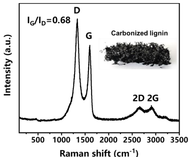
Supplementary Figure 15. Raman spectrum of black charcoal from the pyrolysis of solid lignin at 1400°C for 30 min in N 2 atmosphere.
