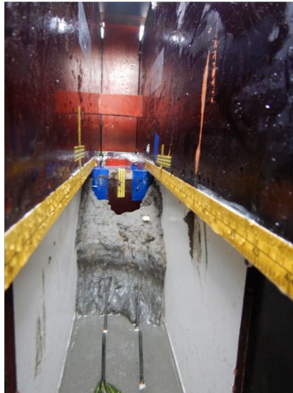
Sandy tidal flat, completely eroded after 3 min of flow exposure
