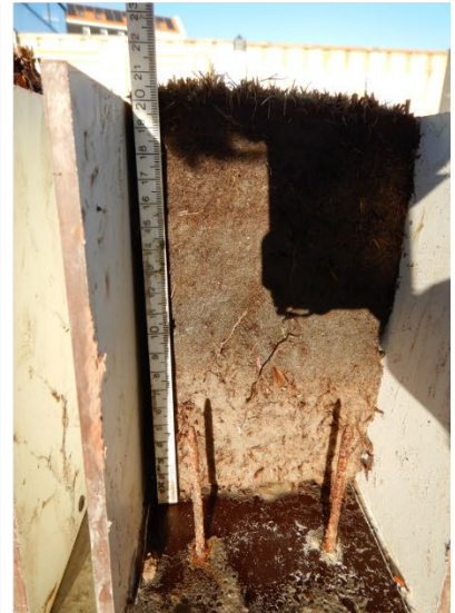
Sandy marsh with cohesive top layer and sandy bottom, not eroded after 3h of flow exposure
