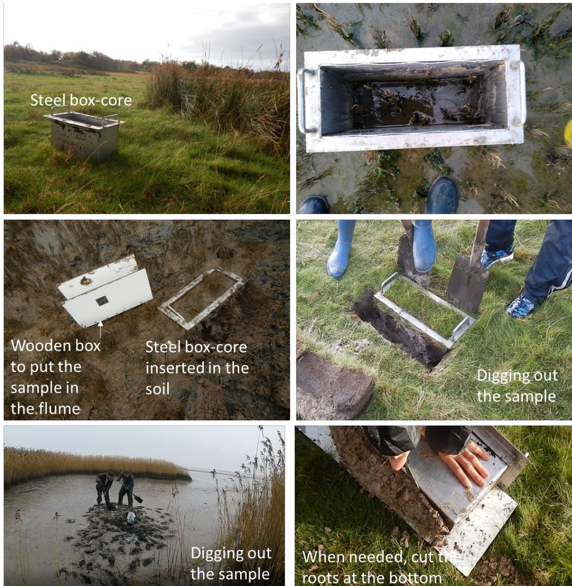
Fig. S1. Images from the method used to collect the rectangular soil samples for the erosion experiment.
