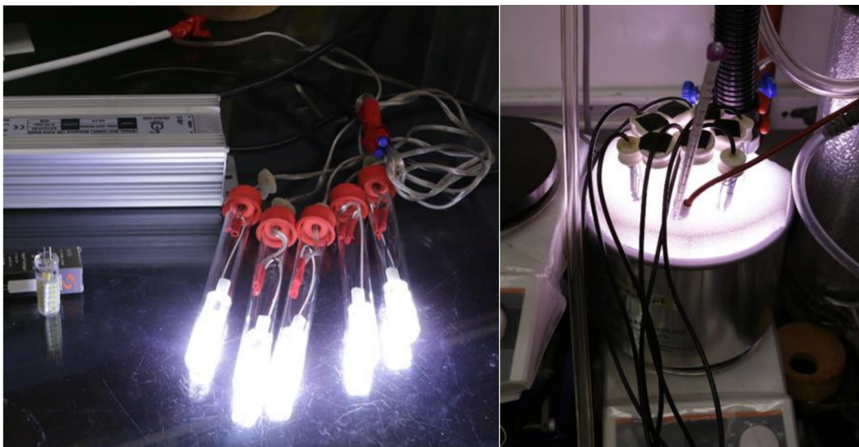
Picture S1. Assembly of LED bulbs from small-scale photochemical reactions.
