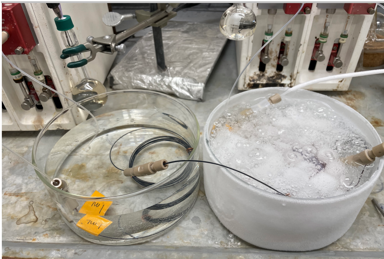
Figure S7. Continuous flow setup for synthesis of bedaquiline 1 . Left reactor coil shows characteristic color of formation of lithiated quinoline 3a in a room temperature water bath. Right reactor coil submerged in IPA/dry ice bath for reaction of 3a with 2 and subsequent reaction quench with MeOH.
