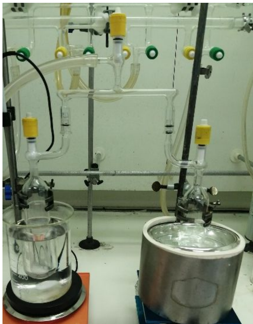
Fig. S36. Vacuum transfer apparatus. From left to right: flask containing polymer and catalyst, T-junction and collection flask
