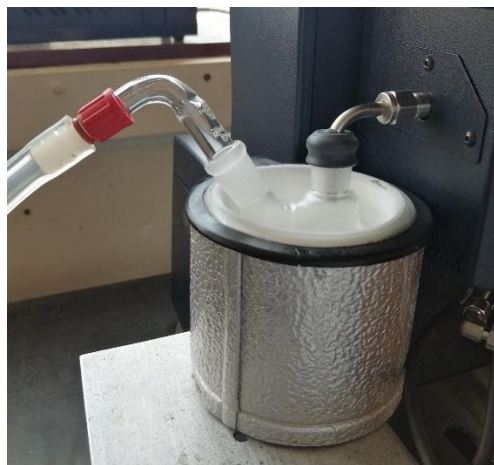
Fig. S4. Experimental apparatus used to isolate the epoxides after the depolymerization reactions on the TGA.
