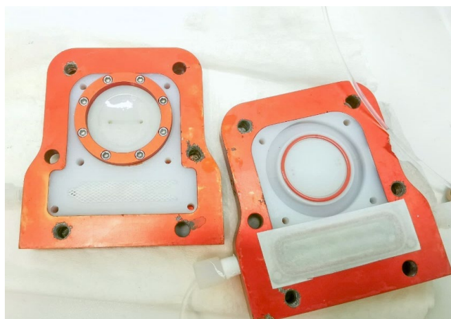
Supplementary Figure 2. Picture of Zaiput SEP-10 used for membrane screening.
