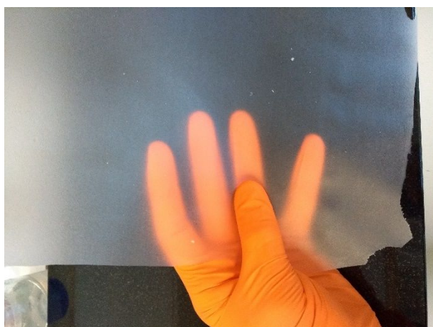
Figure S3 Example of a film obtained by casting a suspension of DAC fibres in water.
