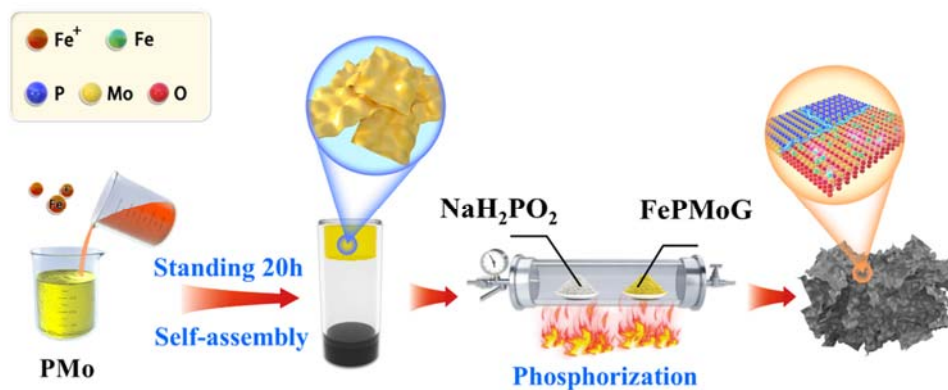
Fig. R11 schematic of synthesis of the Fe/SAs@Mo-based-HNSs electrocatalyst.
