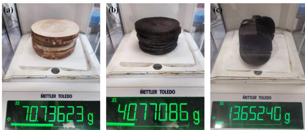
Figure S2. The quality change at different stages of (a) natural wood, (b) stabilization and (c) carbonization process.
