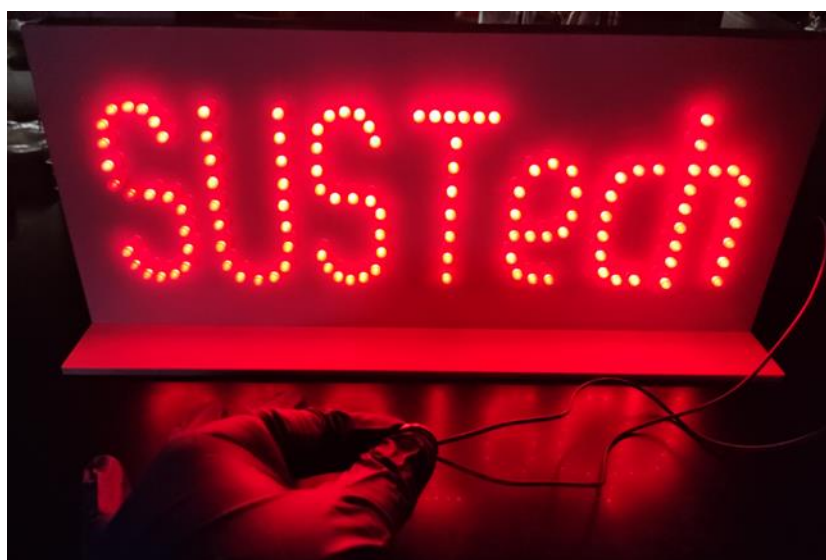
Figure S56. Digital image of an operating LED of SUSTech driven by the high-capacity coin cell.
