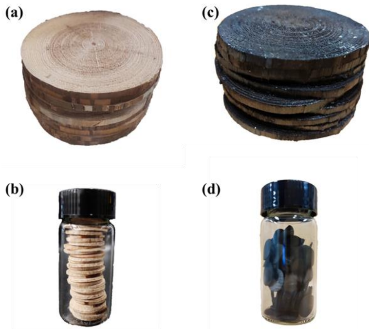
Figure S1. Photographs of (a) the natural wood blocks and (b) after cutting into pieces; (c) the carbonized wood (named MCF) and (d) the MCF pieces.
