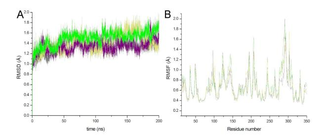
**Fig. S5.** RMSD (A) and RMSF (B) values calculated during the MD simulations of the different proteins studied: PDC-3 (gray), PDC-461 (yellow), PDC-462 (purple) and PDC-463 (green).
