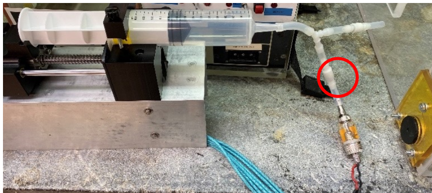
Figure S1. E-cigarette aerosol generation set-up for the collection of condensates. Photograph of the Gram system and the aerosol generation set-up. Red circle indicates the one-way valve where the e-cigarette aerosol condensates are collected.
