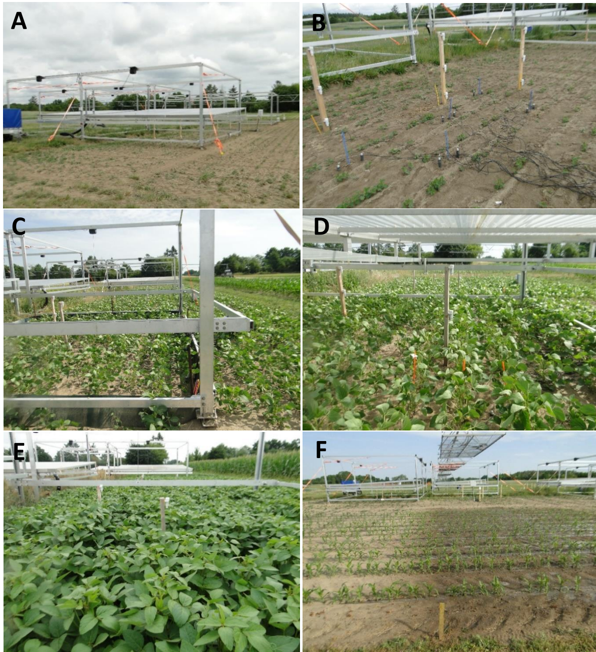
FIGURE S1 | Photographs showing the installation of the rainout-shelter (A), sensors to measure soil and air moisture and temperature on 5 th June 2020 (B); the rainout-shelter in use, open in the front (after it was closed during vegetative stage) and closed in the back at flowering stage (C), one plot in focus with the roof closed at the flowering stage (D) on 29 th June 2021; the rainout-shelter in use, open in the front (after it was closed during vegetative stage) and closed in the back at flowering stage on 21 st July 2021 (E); and a test of the irrigation system on 9 th June 2020 (F). Pictures by G. Rosner/ZALF.
