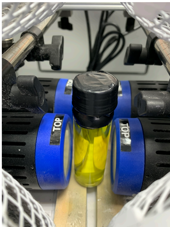
Figure S.3. Arrangement of 60 mL vial for 6.0 mmol scale reactions; reaction appearance prior to irradiation.
