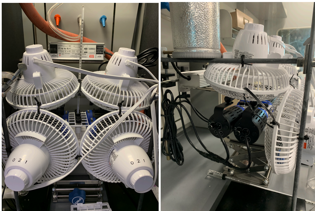
Figure S.1. Reactor cooling fan arrangement. Reactor shown equipped with 7.4 mL vial rack. Front view
