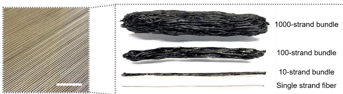
Supplementary Fig. 1 | a , Photograph of meter-long continuous single strand G-LCF. b , Single level G-LCFs deposited on the fiber collector surface and gathered bundle level of G-LCFs with different number of strands. Scale bar, 5 mm.
